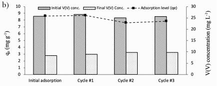
**Fig7.** a) Trials with various adsorbents ranging from Softwood Biochar, RM Wood Biochar and KOH Seaweed hydrochar as examples. b)Effect of regeneration of KOH modified hydrochar ( $HC_{KOH}$ ) on V(V) adsorption level ( $q_e$ ) and on final V(V) concentrations
