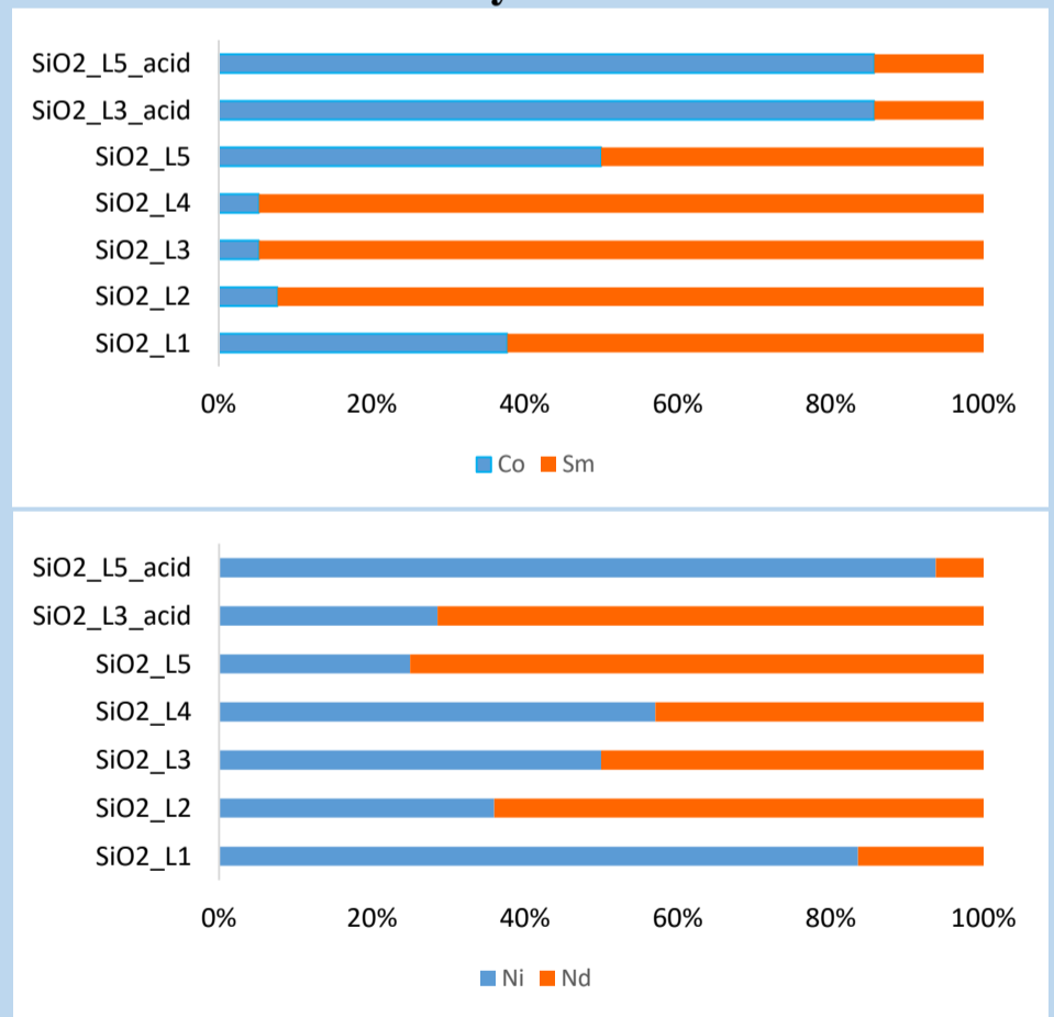
Figure 2. Molar ratios of Co and Ni against Sm and Nd by EDS analysis
