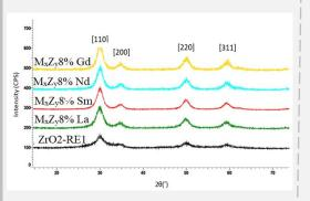
Fig. 1. X-ray diffractograms of the synthesized samples.
