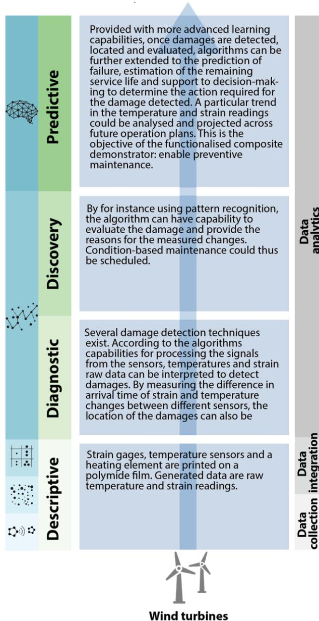
Figure 6: Smart composite for wind turbine safe and efficient operations
